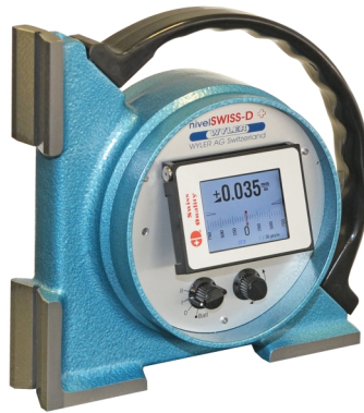
• Digital Nivel Swiss • (formerly NIVELTRONIC) equipped with two prismatic measuring bases in rectangular position to each other for measuring flat surfaces and shafts (diameters \varnothing 20 ... 120 mm) horizontally or vertically. This makes the instrument extremely suitable for adjustments or checks on rectangular geometrical elements of machine tools and structures.
