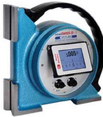
• Digital Nivel Swiss • (formerly NIVELTRONIC) equipped with two prismatic measuring bases in rectangular position to each other for measuring flat surfaces and shafts (diameters Ø 20 ... 120 mm) horizontally or vertically. This makes the instrument extremely suitable for adjustments or checks on rectangular geometrical elements of machine tools and structures.
